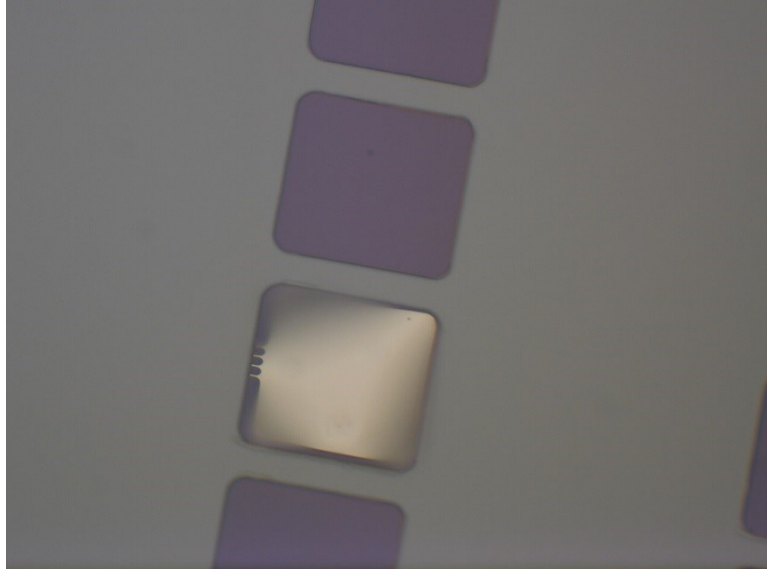
Figure 3.16: Delaminated all-metal hard mask.
