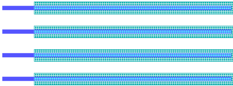
Figure 4.1: Layout with parallel fins. The solid blue is the source metal, and teal as the fin.
