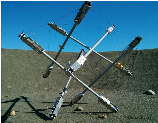
Figure 2.4: SUPERball, an example of a tensegrity robot. The structure of this robot is composed of two primary elements: compression elements (rods) and tension elements (cables).
