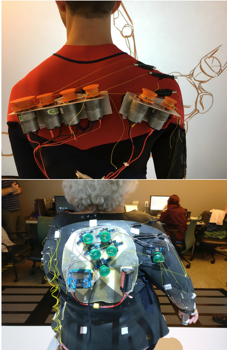
Figure 5.10: Exoskeletal Prototype 1 and 2 (CRUX) viewed from behind. The back-plate on CRUX is more flexible and has greater utility than that on the first prototype [62].
