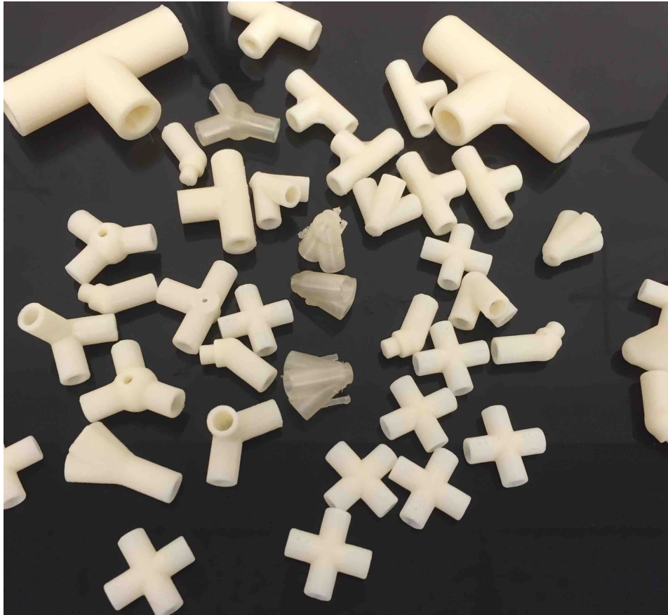
Figure 4.18: Rigid junctions created for connecting rigid components to one another in our tensegrity prototypes. These were crafted via 3D-printing [39].
