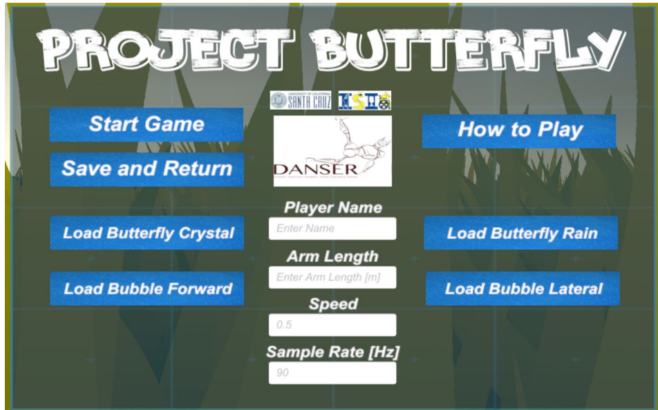
Figure 6.9: A virtual menu used by study proctors to tailor each VR experience towards the specific player [96]. Since player have different dimensions than one another, the game must be adaptable to these differences in order to provide meaningful challenges, irrespective of the user's difference between prior players.
