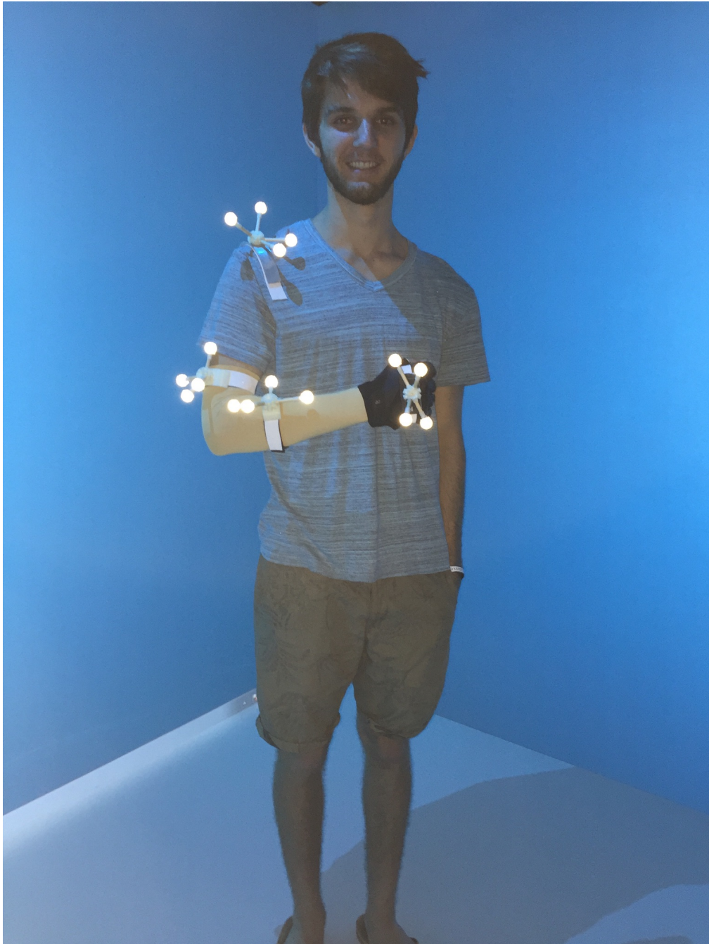
Figure 5.7: The Cave Automatic Virtual Environment (CAVE) for 3D motion capture and virtual reality display. Four cameras in the CAVE track IR-reflective dots, which can be equipped to many materials, including garments.
