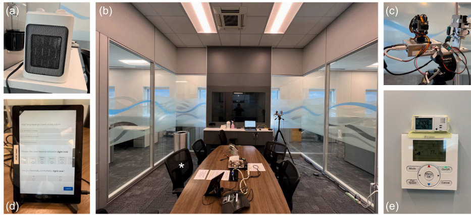
Fig. 4. Demonstration configuration, showing photos of (a) the electric space heater used to simulate a summer heat load; (b) the conference room (about 4.3 m L × 4.3 m W × 3.7 m H), in which the subject’s chair is marked with an asterisk; (c) a close-up of the sensor-controller mounted on a tripod; (d) the survey tablet used to collect thermal sensation and comfort votes; and (e) a temperature/relative humidity logger mounted above the room’s conventional thermostat.
