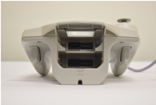
Figure 6.51: Photo of memory+ ports in the center of the front of this Sega Dreamcast default controller
