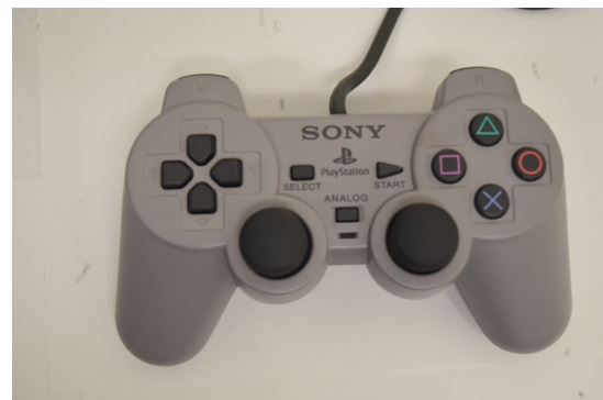
Figure 6.2: Examples of a different style d-pad on the left and two thumbsticks at the lower center of the controller
