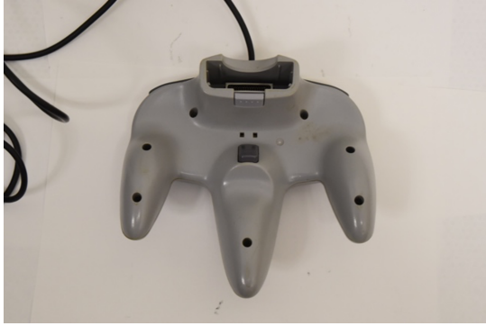
Figure 6.49: Photo of Memory+ port at top middle of the bottom of this Nintendo 64 controller
