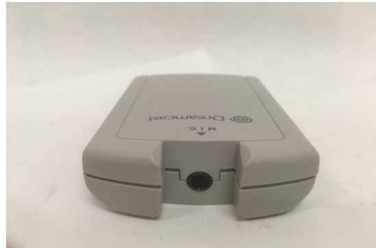
Figure 6.52: Photo of Sega Dreamcast microphone adaptor, or audio/data port adaptor that plugs into memory+ port in Figure 6.51
