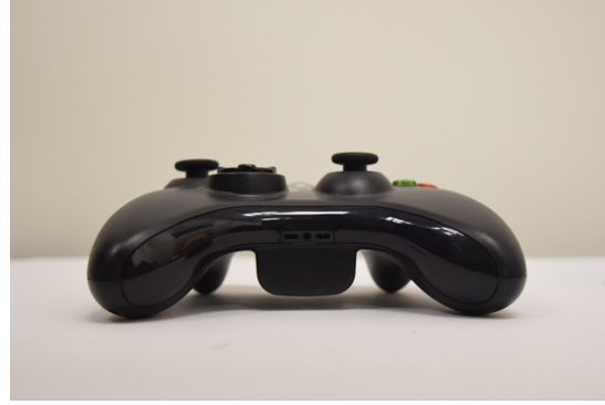
Figure 6.46: Photo of Xbox 360 controller with proprietary audio/data port visible in the center
