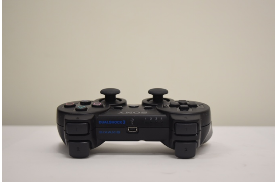
Figure 6.45: Photo of Playstation 3 "sixaxis" controller with charging port visible in the center
