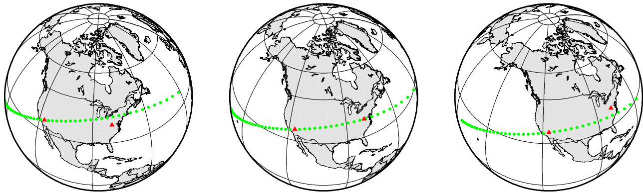
Figure 1. Radar echoes from Mercury sweep over the surface of the Earth during the 2002 May 23 observations. Diagrams show the trajectory of the speckles one hour (left) before, (middle) during, and (right) one hour after the epoch of maximum correlation. Echoes from two receive stations (red triangles) exhibit a strong correlation when the antennas are suitably aligned with the trajectory of the speckles (green dots shown with a 1 s time interval).
