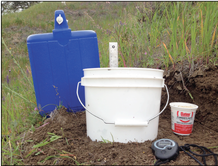
Figure 5: The falling-head single-ring infiltrometer, or bottomless bucket, used to make K_{sat} measurements. Plumber's putty was used to seal the outer edges to prevent leakage. A ruler was attached to the side to measure the rate of infiltration.
