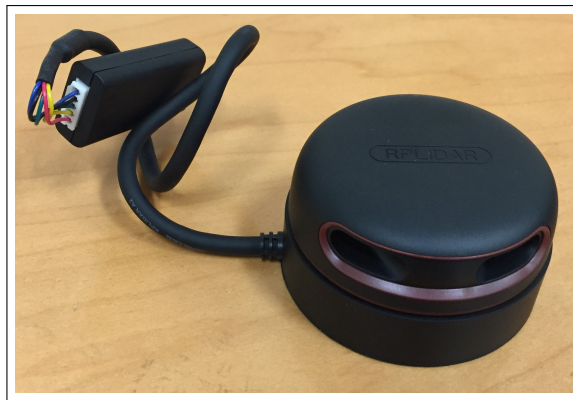
Figure 3.18: The RP LiDAR A2 scans 360 deg with a distance range of 12 meters.
