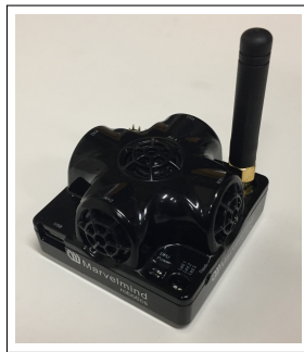
Figure 3.16: The Marvelmind GPS kit is designed to provide \pm 2 cm accuracy for indoor navigation.
