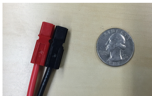
Figure 3.28: Anderson power pole
