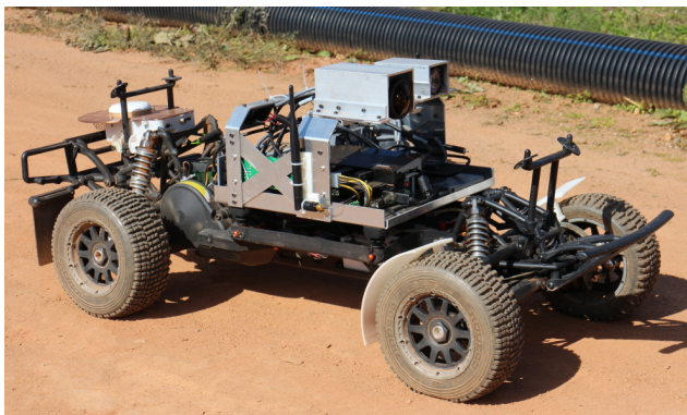
Figure 3.5: The AutoRally Robot is a testbed for perception and control from the Georgia Institute of Technology. Image from [20].
