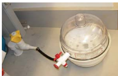
Fig. 2-2. Desiccator attached to a vacuum
