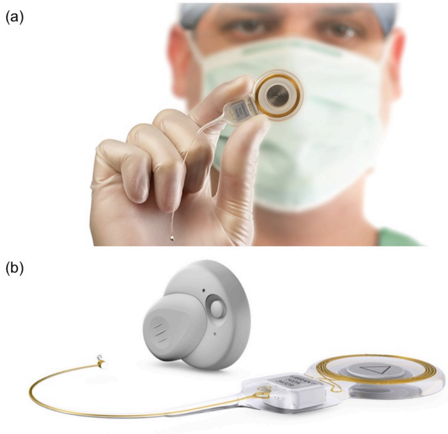
Fig. 14 Vibrant Soundbridge middle ear implant components 66 (a) actual image of the internal components of the VSB that is implanted under the skin with the FMT attached to the long process of the incus (b) actual image of both external and internal components of the VSB middle ear implant system. (Image courtesy of MED-EL GmbH, reused with permission)
