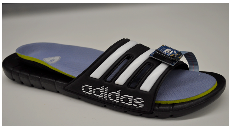
Fig. 98 StabilitySole Insole placed in a shoe. This first prototype used a wireless data transfer system. Later models utilized a data logging system that was more power efficient and size appropriate.
