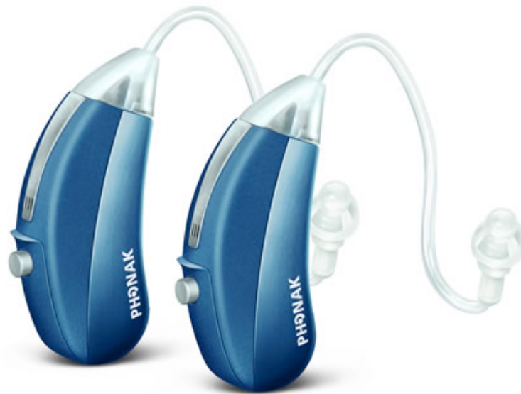
Fig. 5 Mini behind-the-ear (BTE) hearing aid, the 'Milo' by Phonak 33 .
