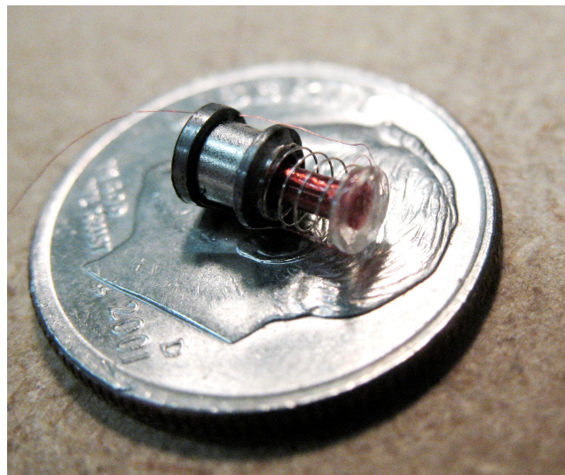
Fig. 29 DHD actuator components a) inner flux guide b) outer flux guide c) spring d) inner flux guide, permanent magnet, and outer flux guide assembly e) assembly in part d with spring added f) fully assembled actuator with micro holes drilled in the outer and inner flux guides to allow for the voice coil leads to be protected during operation
