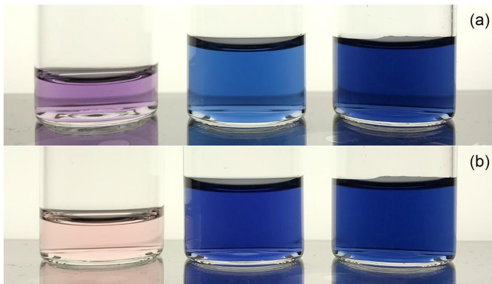
Figure 6.10. Supernatant of the blue AgNP solution, a solution with the pellet re-dispersed in 1.5 mM \text{Na}_3\text{Cit} , and the as-prepared AgNP solution (left to right). Centrifugation for 15 minutes at (a) 10,000 rpm and (b) 17,500 rpm.
