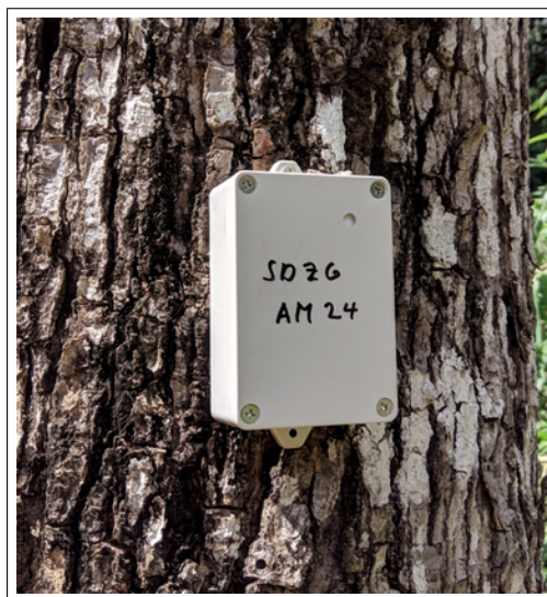
Figure 1.5. Madre de Dios, Peru Audiomoth Deployment Tree Attachment Example
