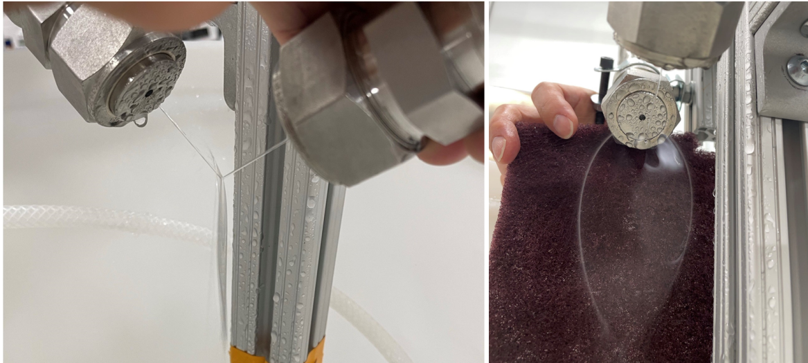
Figure 7. Water film produced by colliding two jets from 1-mm diameter nozzles.
