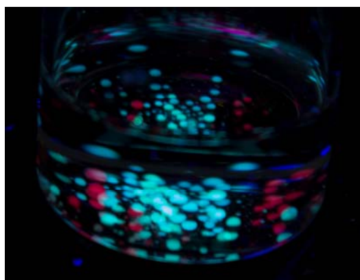
Figure 6.12 V50/FP hydrogel beads. The photograph shows turquoise, green and red beads illuminated by long range UV light.
