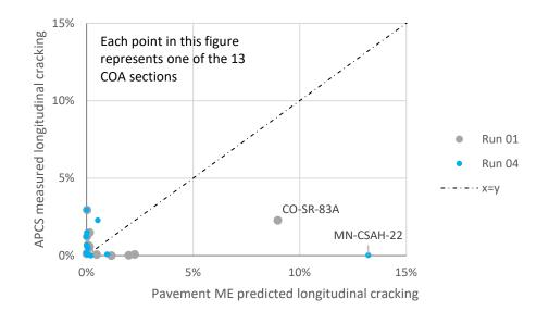
Figure 4.4: Comparison between Run 04 predictions (50% reliability) and measured cracking (Run 04 LTE is based on FWD testing).
