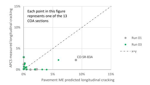
Figure 4.3: Comparison between Run 03 predictions (50% reliability) and measured cracking (Run 03 MR<sub>28-day</sub> is based on laboratory testing of actual concrete).
