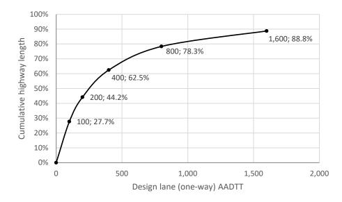
Figure 2.1: Truck volume in Caltrans's non-interstate highway network.
