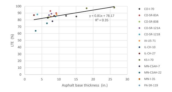
Figure 4.5: Comparison between LTE measured with FWD and thickness of asphalt measured from cores.
