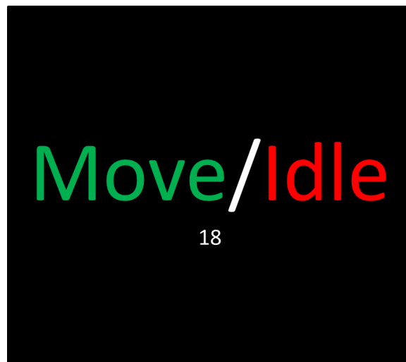
Figure 2.3: Example interface for the offline training session for BCI systems using textual cues with visual feedback applied after each trial, in this instance, after each “Idle” or “Move” trial.
