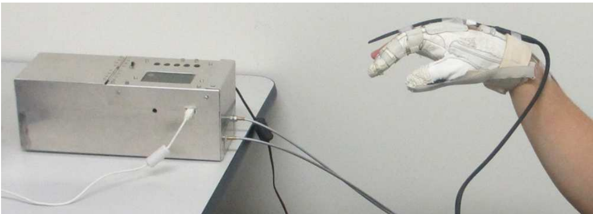
Figure 3.2: Image of the hand orthosis [102] used in the study [78, 83].
