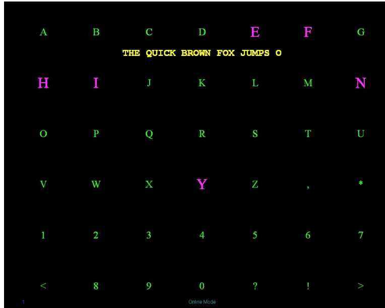
Figure 1.6: Screen capture showing the matrix of characters in the P300 speller interface [148]. The illuminated characters are bold-faced and highlighted in pink. The typing prompt (yellow) shows the spelling progress.
