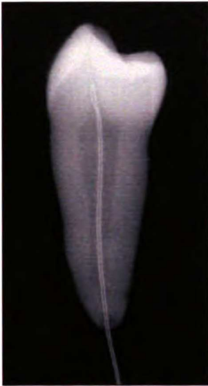
Figure 1. Radiographic image of extracted human bicuspid with thermocouple inserted up through the apex into the most occluso-facial aspect of the pulp horn.
