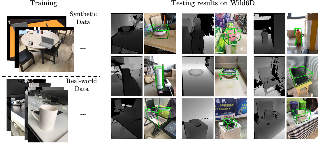
Figure 4.1. Left: we train our model with both synthetic data and real-world data under our proposed semi-supervised setting. Right: during inference, given the RGBD images, the object pose can be estimated precisely. Green 3D bounding boxes denote the ground truth, and the red boxes are estimation results via our proposed method
