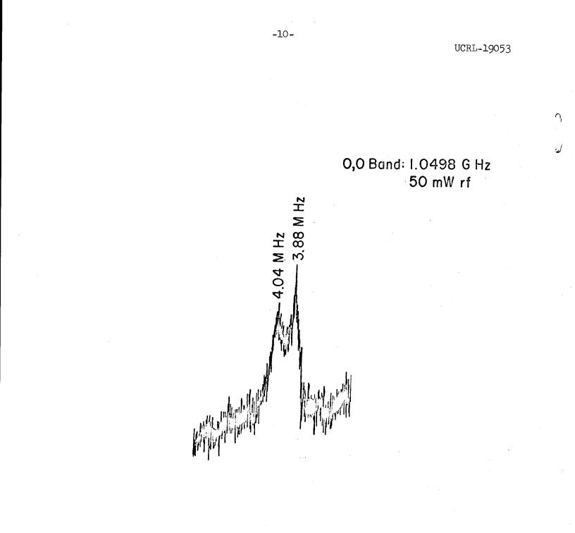
Figure 1: Optically detected ENDOR transition at 3.96 MHz while saturating the 1.0498 GHz microwave transition.
