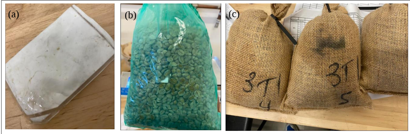
Figure 2.5. Liquified \text{CaCl}_2 in \text{CaCl}_2 treatments. a) \text{CaCl}_2 leakage from desiccant pack. b) \text{CaCl}_2 leakage into a coffee sample in a GP-Bag. c) \text{CaCl}_2 leakage through the jute sack of a jute sack with desiccant ( \text{CaCl}_2 ) treatment.
