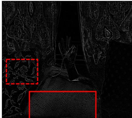
Figure 3.10: Comparison of feature detection using smooth derivative operator to the case of feature detection using Phase Stretch Transform (PST). Original image is shown in (A). Smooth derivative operator is unable to efficiently visualize the low contrast details in the dark areas of the image. However, PST captures these contrast changes in low-light-level areas due to its intrinsic equalization property.
