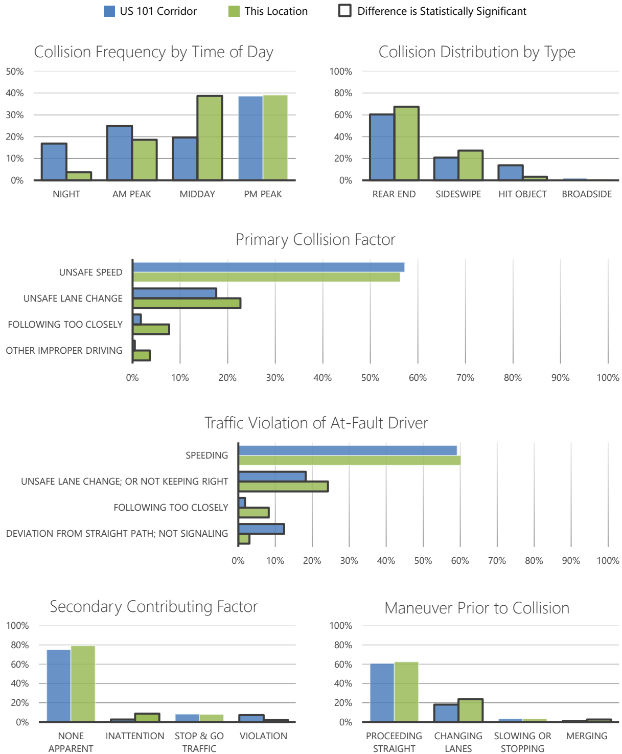
Figure A-3: Northbound Crash Hotspot #2: Incident Data Approaching Potrero Ave Junction
