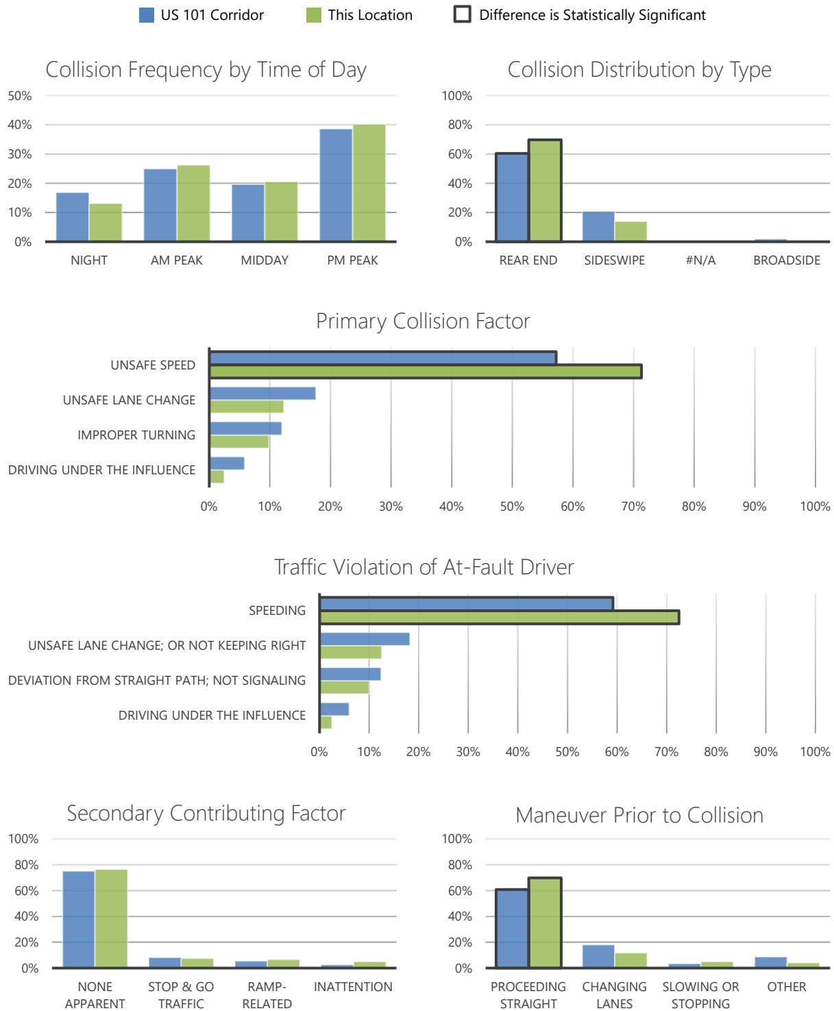
Figure A-7: Northbound Crash Hotspot #6: Incident Data at San Antonio Rd
