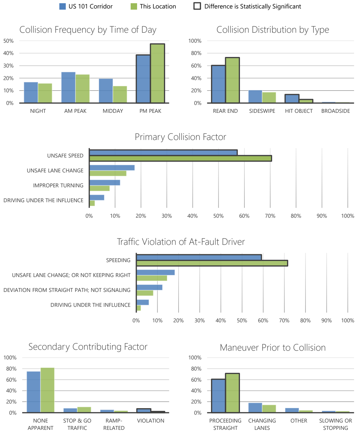
Figure A-11: Southbound Crash Hotspot #4: Incident Data at San Antonio Rd
