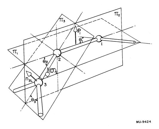
Fig. 2. Schematic diagram of the scattering planes in the measurement of the rotation parameter R.
