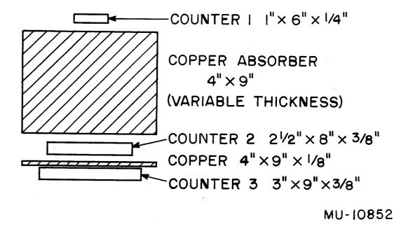
Fig. 3. Scale drawing of the three counter telescope used for the double scattering measurements.
