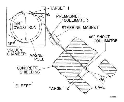
Fig. 1. Plan view of the cyclotron and orbit of the polarized beam. If the cyclotron is viewed from above the spins of the polarized beam is upward.
