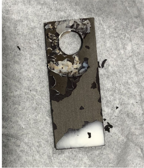
Figure 4.3: Extreme flaking observed from a 316SS sample exposed to 650°C Solar Salt during post-extraction storage.
