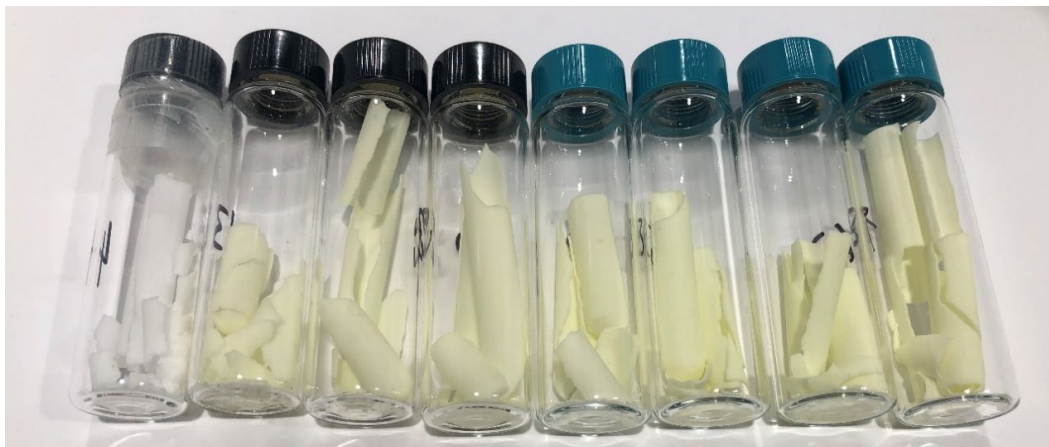
Figure 5.67: Solid nitrate salt samples taken from 600°C experiment from left to right: after initial bakeout, 500hr, 1000hr, 1000hr fresh salt bakeout, 2000hr, 3000hr, 4000hr, and 5000hr.
