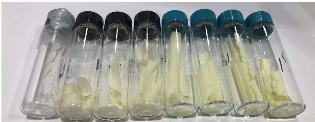
Figure 5.66: Solid nitrate salt samples taken from 590°C experiment from left to right: after initial bakeout, 500hr, 1000hr, 1000hr fresh salt bakeout, 2000hr, 3000hr, 4000hr, and 5000hr.
