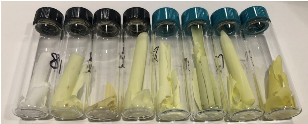
Figure 5.69: Solid nitrate salt samples taken from 630°C experiment from left to right: after initial bakeout, 500hr, 1000hr, 1000hr fresh salt bakeout, 2000hr, 3000hr, 4000hr, and 5000hr.
