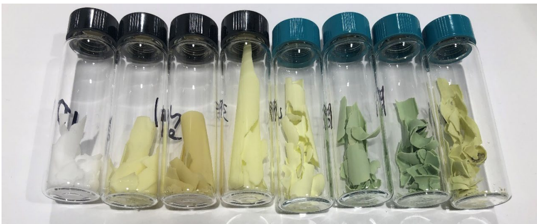
Figure 5.70: Solid nitrate salt samples taken from 650°C experiment from left to right: after initial bakeout, 500hr, 1000hr, 1000hr fresh salt bakeout, 2000hr, 3000hr, 4000hr, and 5000hr.
