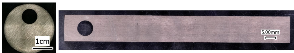
Figure 3.3: Examples of the coupon dimensions for experiment set 1. Left: 1-inch diameter sample machined from N60 rod. Right: 10cm sample machined from sheet.
