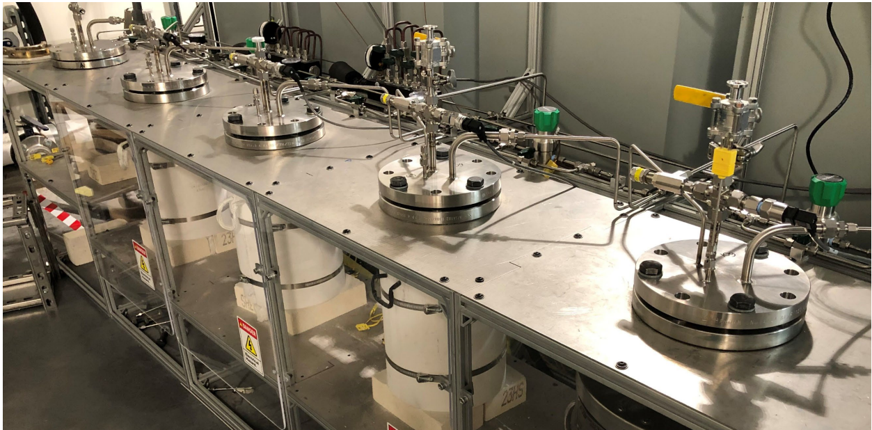
Figure 3.1: Five duplicate corrosion vessels utilized for Solar Salt corrosion experiments.
