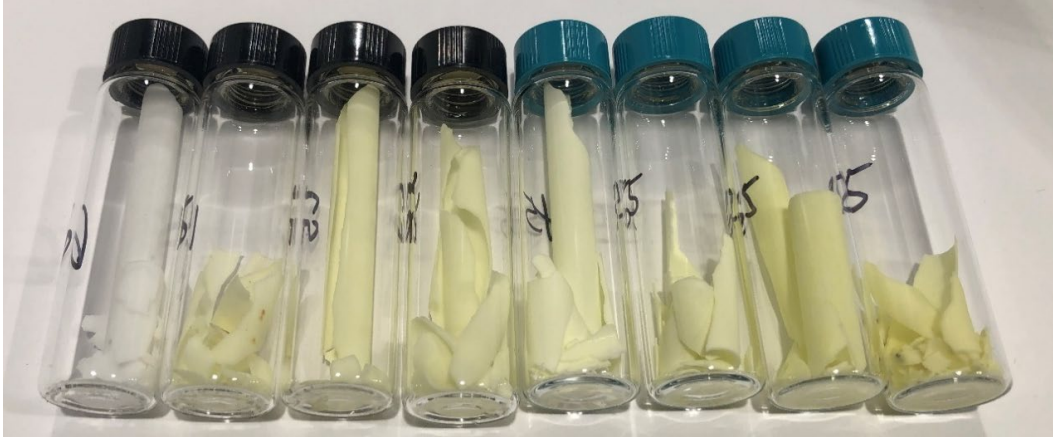
Figure 5.68: Solid nitrate salt samples taken from 620°C experiment from left to right: after initial bakeout, 500hr, 1000hr, 1000hr fresh salt bakeout, 2000hr, 3000hr, 4000hr, and 5000hr.
