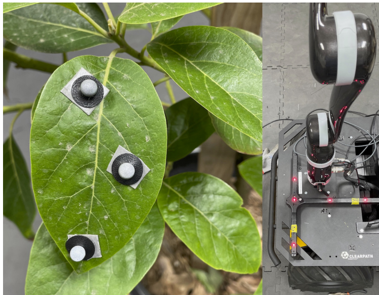
Figure 3.7: We used motion capture to establish a ground truth for determining the leaf 6D pose. Markers were placed on a target leaf (left) with origin at the base of our 6-DOF robot (right). (A real avocado tree was used.)
