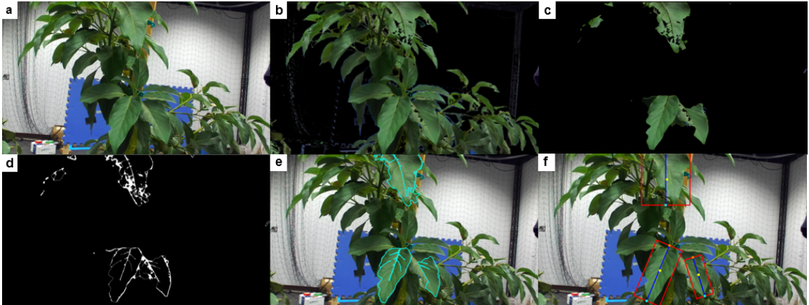
Figure 3.2: Key instances and operations of the proposed 2D leaf detection algorithm. (a) Original RGB left image, (b) Threshold segmentation, (c) Depth segmentation, (d) Canny edge detection, (e) Contour detection, (f) Output bounding boxes and annotated keypoints.
