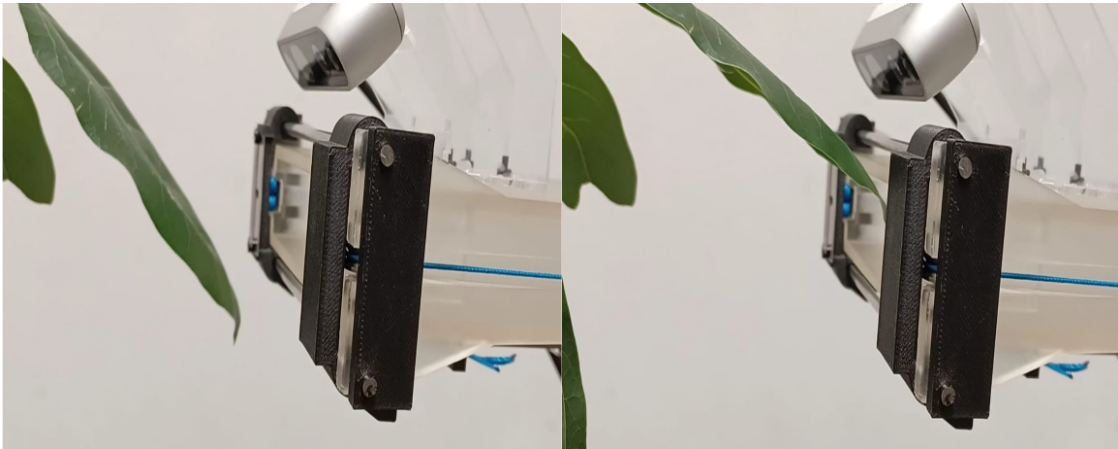
Figure 3.14: Effect of the air suction mechanism on a leaf. The end-effector secures the tip of the leaf, allowing it to be captured even if the end-effector is misaligned or some misplacement is caused, e.g., by wind.
