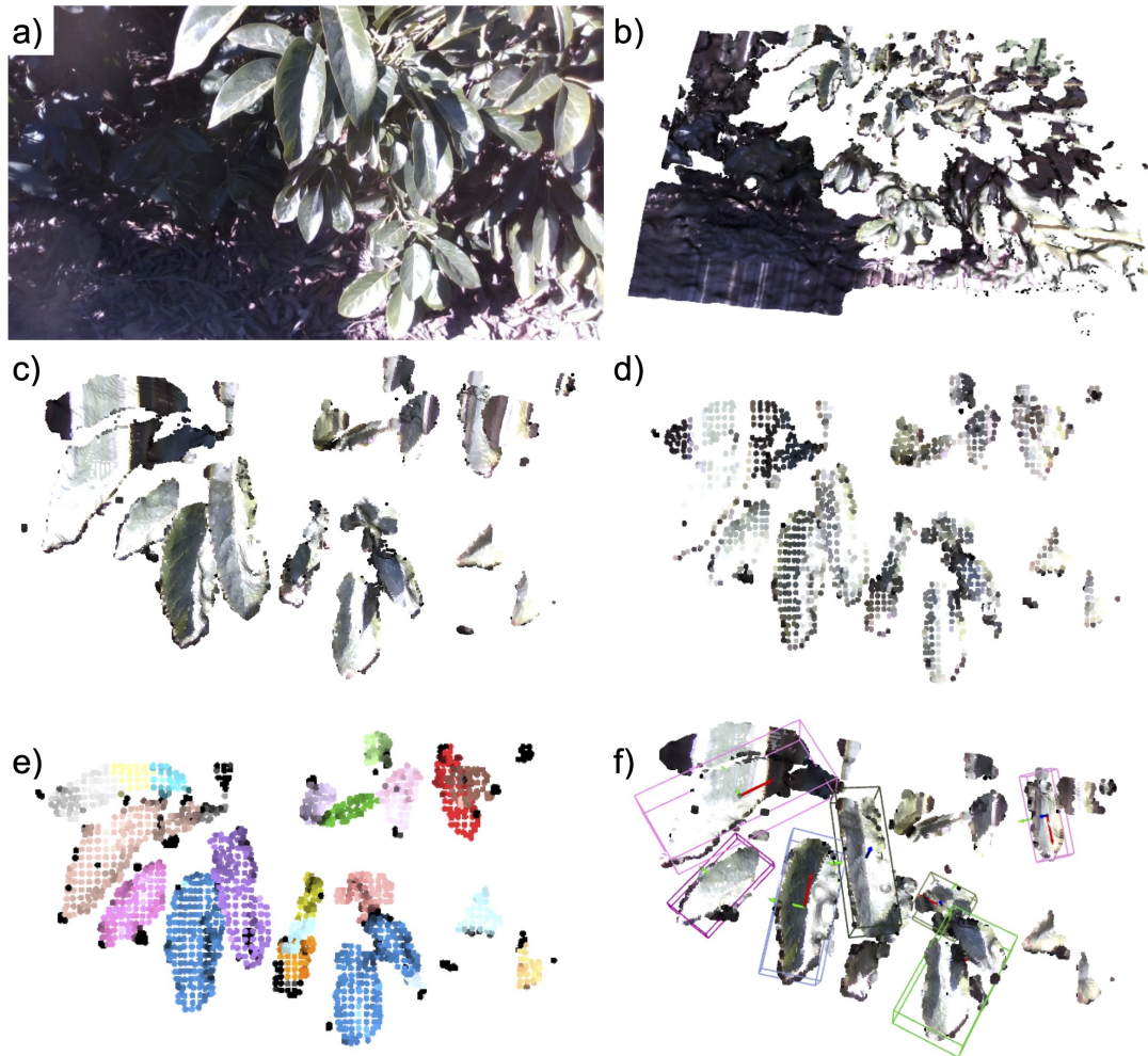
Figure 3.6: Key steps in our proposed leaf detection and localization process. The sample here corresponds to an outdoor point cloud: (a) corresponding RGB image of the tree, (b) raw point cloud, (c) distance filtered ROI, (d) downsampled point cloud, (e) segmented clusters, and (f) detected candidate leaves without 6D pose bounding boxes.
