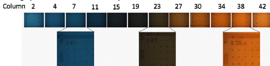
Figure 10. Representation of the gradient over the microwell array using food dye.
