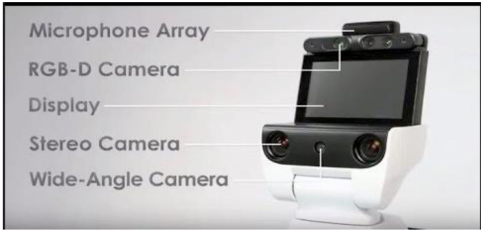
Figure 7: HSR Placement of Cameras and Microphones Source: Toyota Motor Corporation (Toyota 2015)
