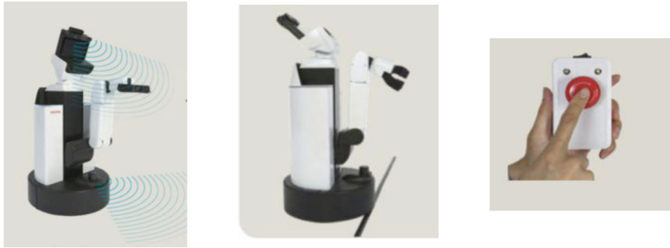
Figure 9: Safety Feature—Obstacle Avoidance Sensors; Magnetic Tape Barriers; Hand-Held STOP Button
