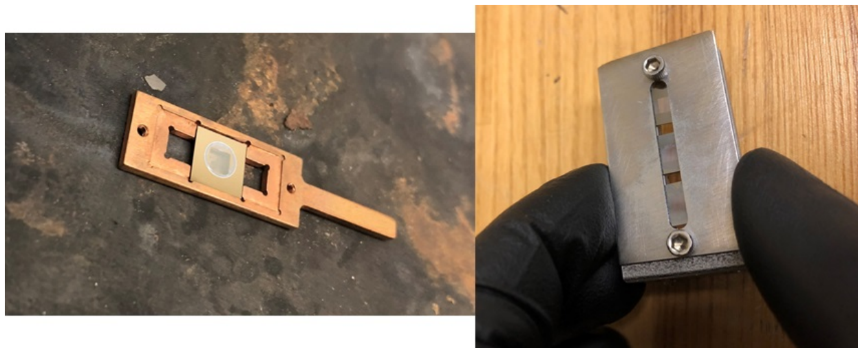
Figure 5.1: The sample is drop-cast and dried in atmosphere on a silicon nitride window. The samples are held in a holder that sandwiches the edges and allows for simultaneous static spectra to be taken for the NV, P1, and a blank sample.
