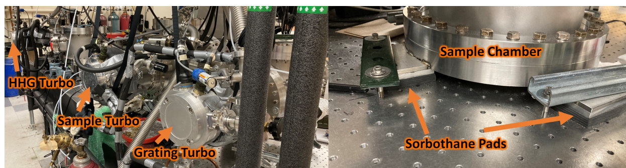
Figure 2.8: Photographs of the turbomolecular pumps, which introduced significant timing jitter are shown on the left. The simple solution of a rubber pad underneath the vacuum chambers is shown on the right.
