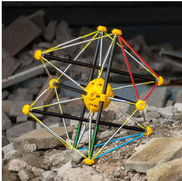
Figure 3.2: Tensegrity structure with highlighted closed face (red), open face (blue) and double rod (green) landing orientations
