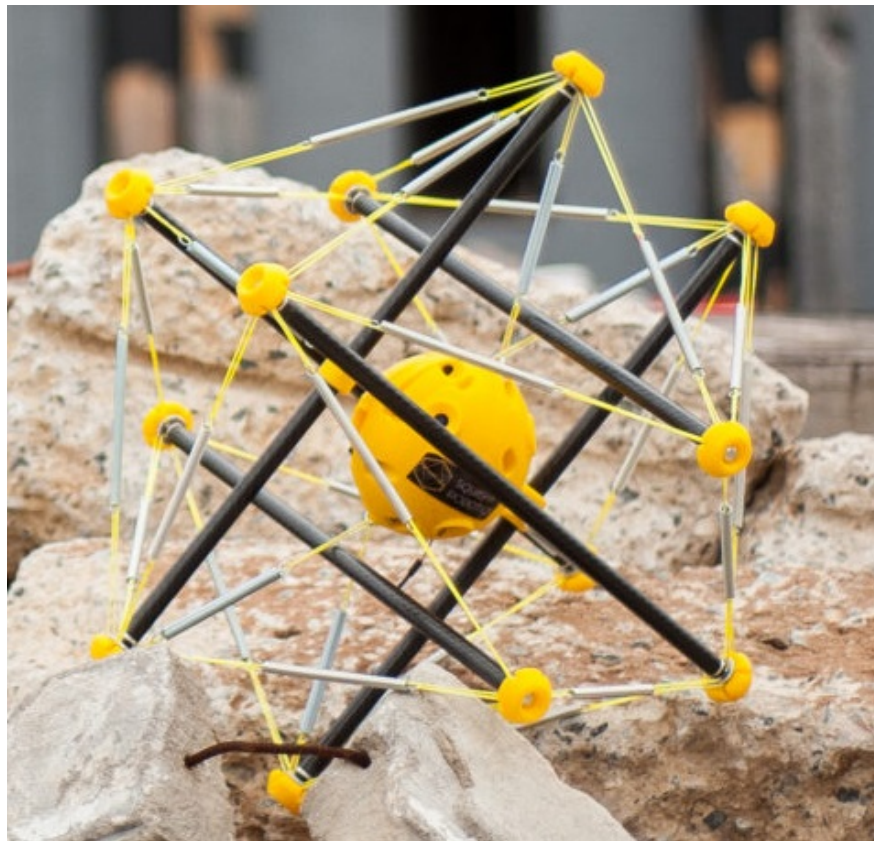
Figure 2.4: Squishy Robotics stationary robot in a simulated disaster environment
