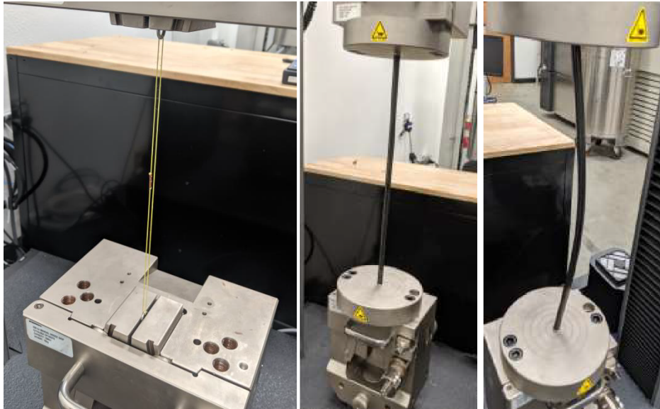
Figure 2.5: From left: Cable pull test setup, rod compression test setup, rod buckling after loading. Photos courtesy of NTS.
