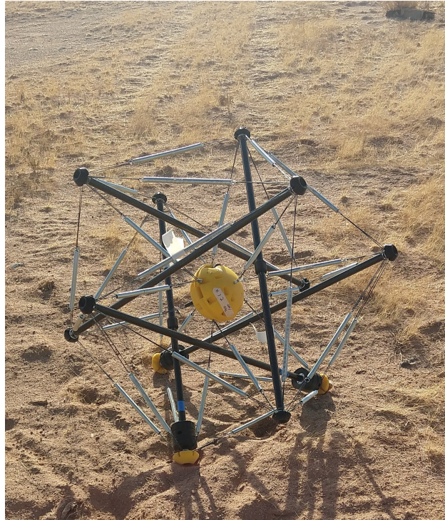
Figure 5.8: 30" robot correctly oriented after cargo plane drop test
