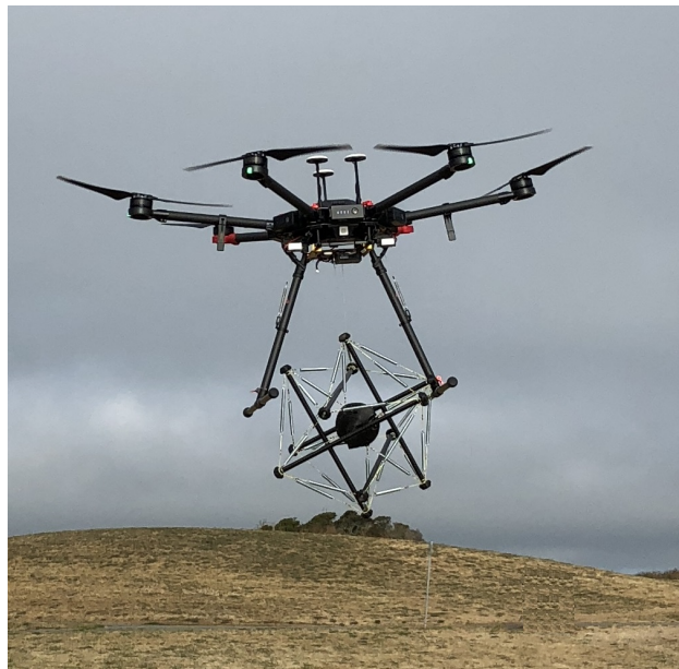
Figure 4.4: Drone drop test of tensegrity lander
