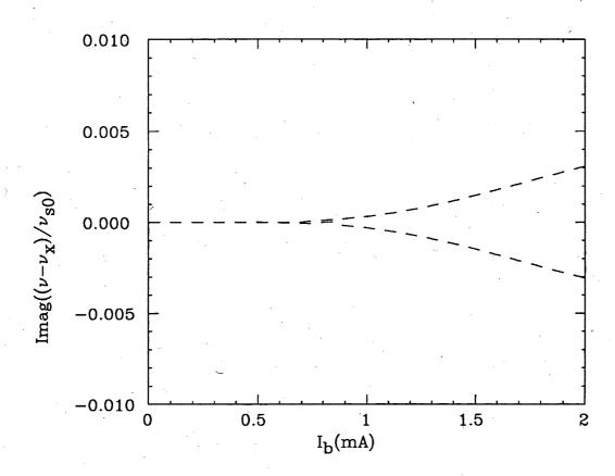
Figure 4: Imaginary parts of  $(\nu - \nu_x)/\nu_{s0}$  in the double rf system.  $\sigma_{\phi 0} R/h = 13.12$ cm.
