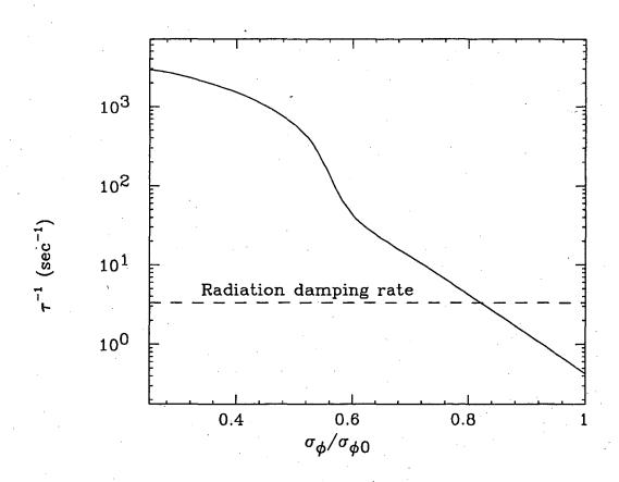
Figure 7: Growth rate  $\tau^{-1}$  at  $I_b=0.75 \mathrm{mA}$  as a function of the bunch length  $\sigma_\phi$  in units of  $\sigma_{\phi 0}$  where  $\sigma_{\phi 0} R/h=13.12 \mathrm{cm}$  is the original bunch length.
