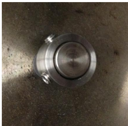
Figure 11. Nickel sample mounted in top of oxide removal autoclave
