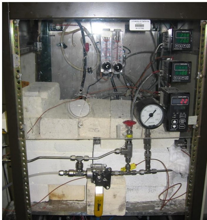
Figure 5. Assembled front of stainless steel autoclave
