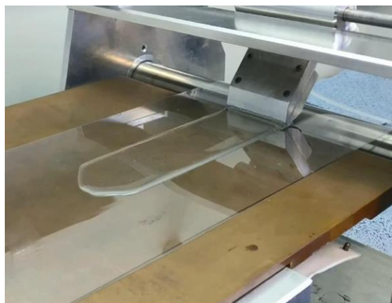
Figure 1.4: Picture depicting the slot-die apparatus used by Premble et al. to extrude continuous chitosan thin films[13].
