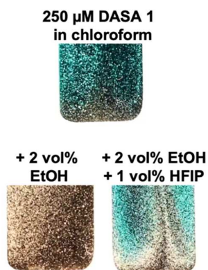
Figure 4.42. photographic stills of video 1 of 250 \mu\text{M} DASA-3 in chloroform with either no addition, 2 vol% ethanol and 2 vol% ethanol and 1 vol% HFIP under irradiation with white light.
