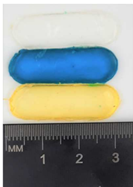
Figure 6.9. Dimensions of films 1-3 on the polydomain after being taken out of the molds.
