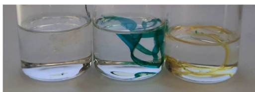
Figure 6.13. Swelling of Films 1-3 in DCM. Gel fraction obtained after 24 hrs in DCM
