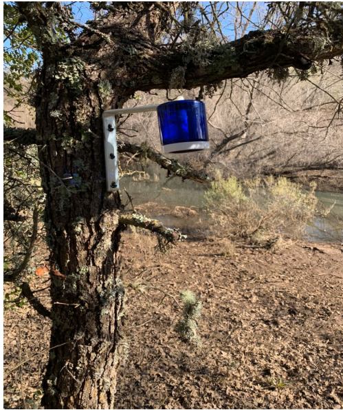
Figure 5: An example of the installation of the MerPAS, depicted at NAMD. This photo and approach were developed by Straw (2023) 44 . Alongside every shield, 2 air collectors were installed approximately 1.5 m off the ground and left in the field for about 60 days.
