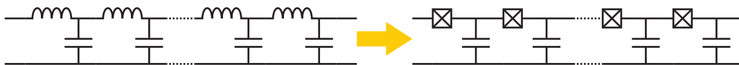
Figure 4.6: “LC ladder” lumped-element transmission line, and equivalent nonlinear lumped-element transmission line utilizing the Josephson inductance.
