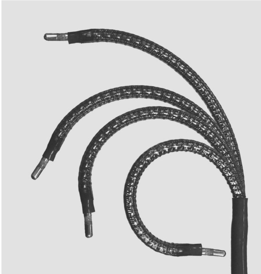
Figure 1.2. This figure, which originally appeared in Camarillo et al. [5], depicts a tendon driven continuum manipulator. These types of robots are unique in that they possess infinite degrees of freedom in the continuously varying curvature of their flexible backbones.
