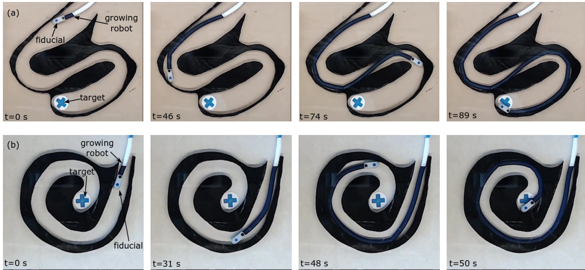
Figure 3.5. Time-series images of a growing robot with a ring magnet at its tip as it extends through constrained paths resembling (a) an “S” and (b) a spiral. In each scenario, the robot must conform to the curvature of the path in order to reach the target at the end, marked with a blue X.
