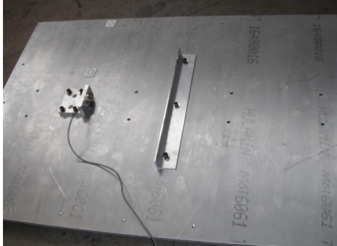
Figure 2-13: Omega 500 lb. button style excavation load cell. The load cell is mounted on the bottom side of the soil bin plate and contacts the driver carriage, reference Figure 2-6.
