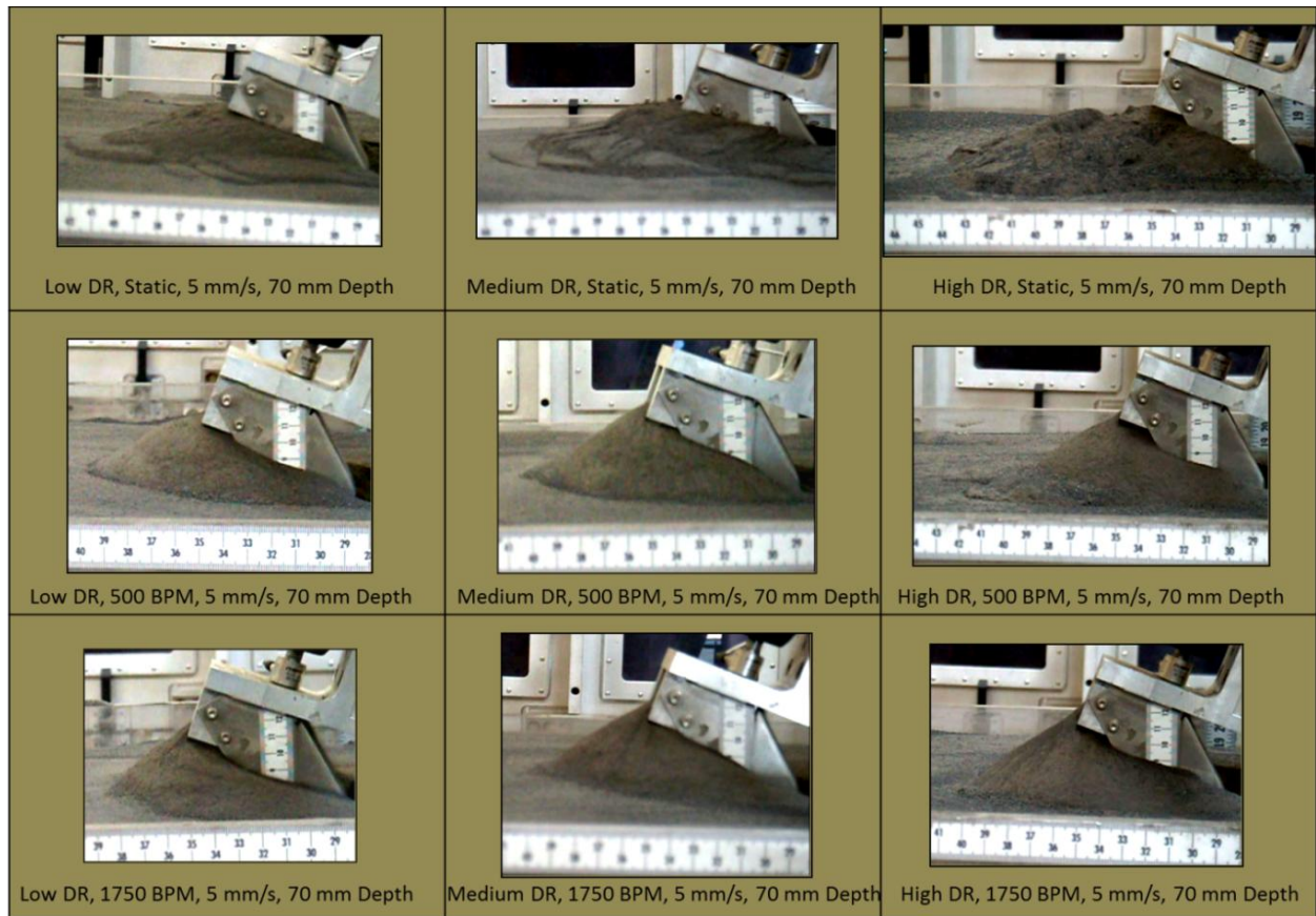
Figure 5-26: Graphic of physical change in shape of failure boundary geometry during excavation.
