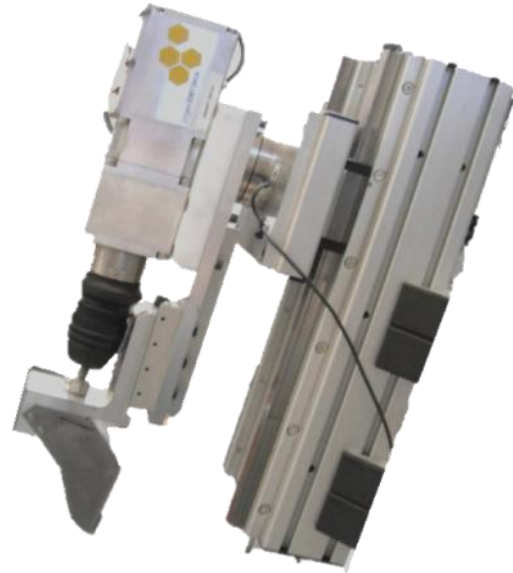
Figure 2-12: ATI Mini 85 Six Axis Force and Torque Load Cell rigidly fixed to the digging axis bearing rail and the percussive mechanism.
