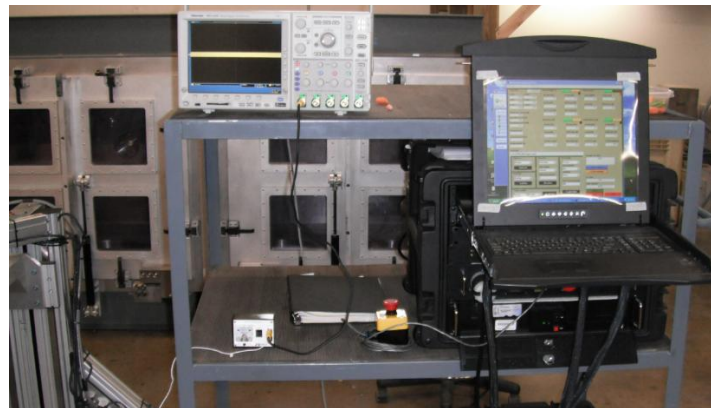
Figure 2-17: Data acquisition system: Honeybee Robotics control module, ATI data acquisition software, and oscilloscope.
