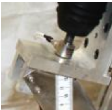
Figure 2-14: Piezo load cell mounted between the excavation scoop and the impact rod.
