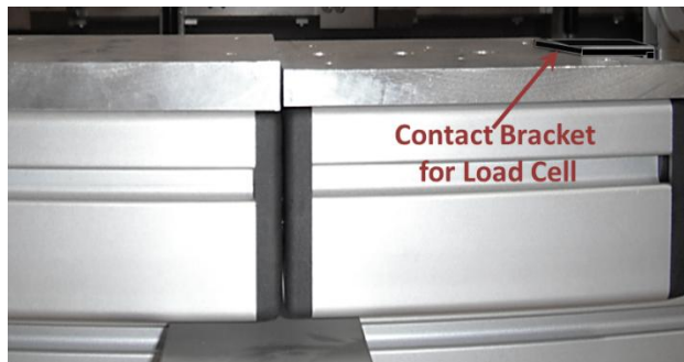
Figure 2-7: The difference in height between carriage #2 and #3; the follower carriage and the driver carriage. Load cell interaction bracket shown on driver carriage.
