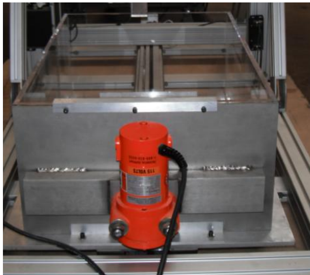
Figure 2-9: External vibrator used for soil compaction.
