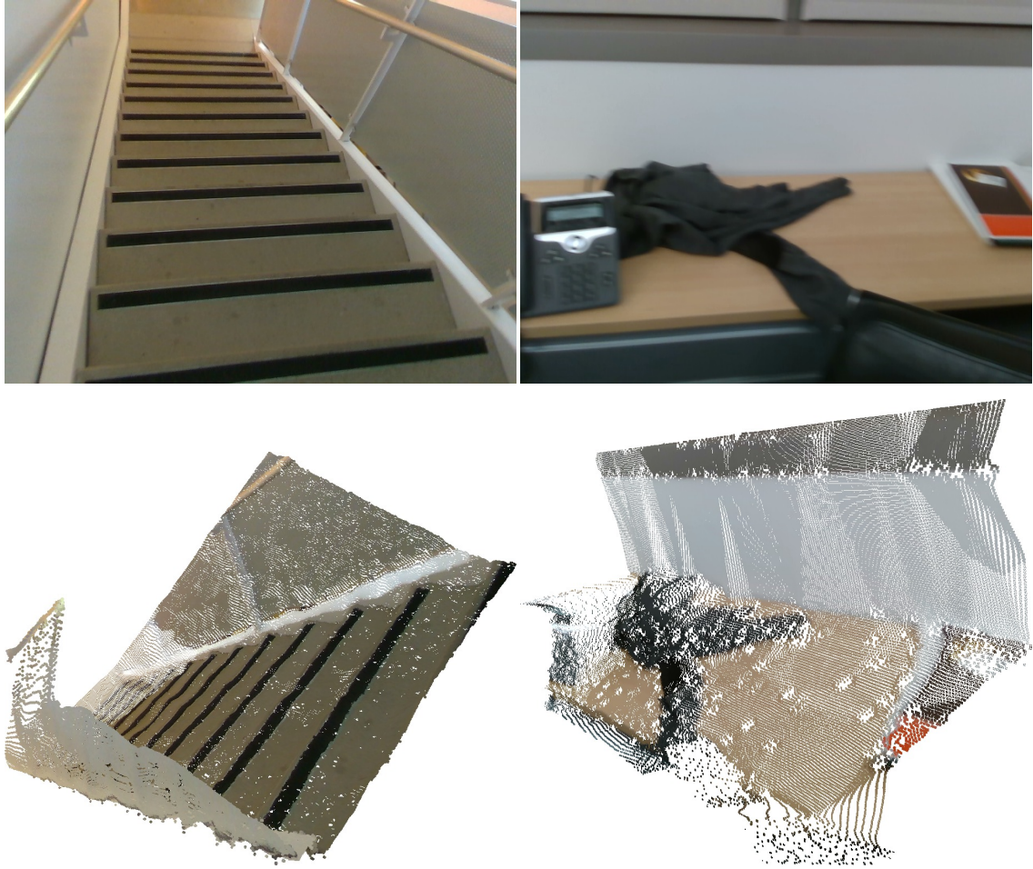
Figure 5.6: Qualitative evaluation on VOID benchmark. Top: Input RGB images. Bottom: Densified depth images back-projected to 3D, colored, and viewed from a different vantage point.
