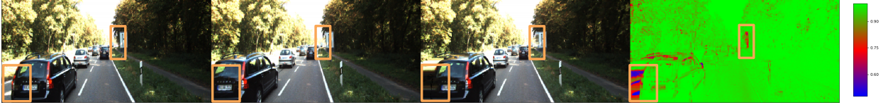
Figure 2.1: Examples of our adaptive weighting scheme as images. Left to right: left image, right image, left reconstruction, adaptive weights. The adaptive weights reduce regularization at regions of high residual; hence, they discount dis-occlusions and occlusions as in the highlighted regions.
