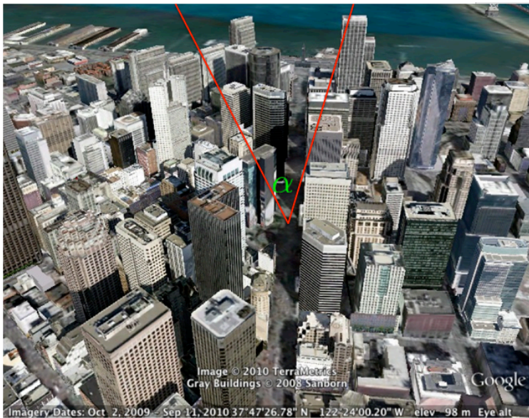
Figure 10 Mask-Angle Representation using street width and building heights
