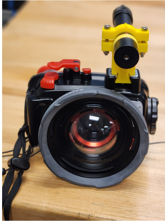
Figure 2.1. A fully assembled FishSense Lite hardware unit.
