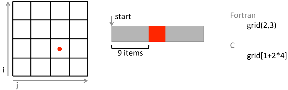
Figure 8.6: Left: Logical view of a 2D grid that holds scalar values, with a point highlighted in red. Center: View from the perspective of memory for the highlighted red location. Note that in memory, the grid is simply a flat 1D memory array. Right: Accessing the highlighted point in Fortran and C. Although C supports multidimensional arrays, the implementation is inefficient due to the large amount of “pointer chasing” incurred. Thus, structured grid computations usually mimic the Fortran model of multidimensional arrays by creating a flat 1D array and explicitly calculating offsets.
