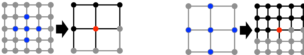
Figure 8.8: The restriction and prolongation operators used in multigrid, both of which are implemented as structured grid kernels. Left: Restriction operator on a 2D grid. Points in the coarser grid depend on fine grid points, with some kind of weighted averaging used in the translation. Right: Prolongation operator. Another set of weighted averages translates data from the coarse grid to the finer one.
