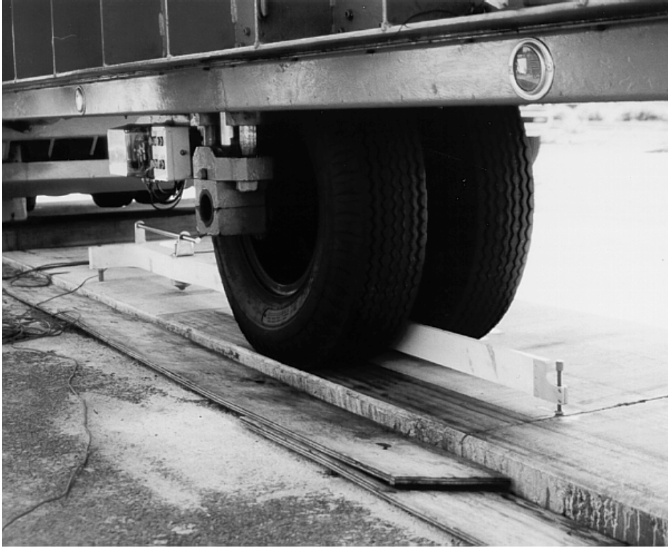
Figure 19. Road Surface Deflectometer.
