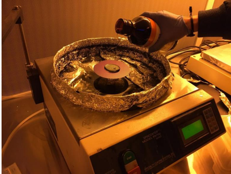
Figure 24: The spin coating for SU-8 2015
