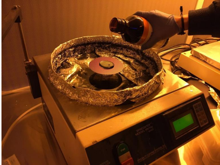
Figure 24: The spin coating for SU-8 2015
