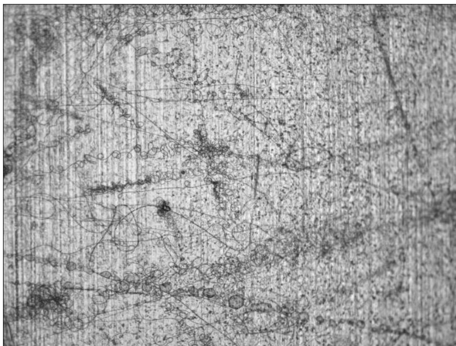
Figure 12: The image of the deposited 10% PAN obtained by the in-house far-field electrospinning
