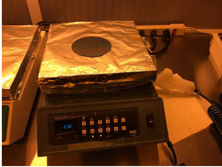
Figure 25: Soft-bake of coated silicon wafer
