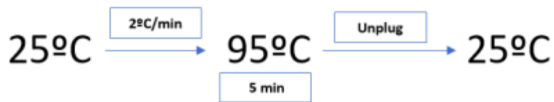
Figure 26: Temperature Ramp used for soft bake
