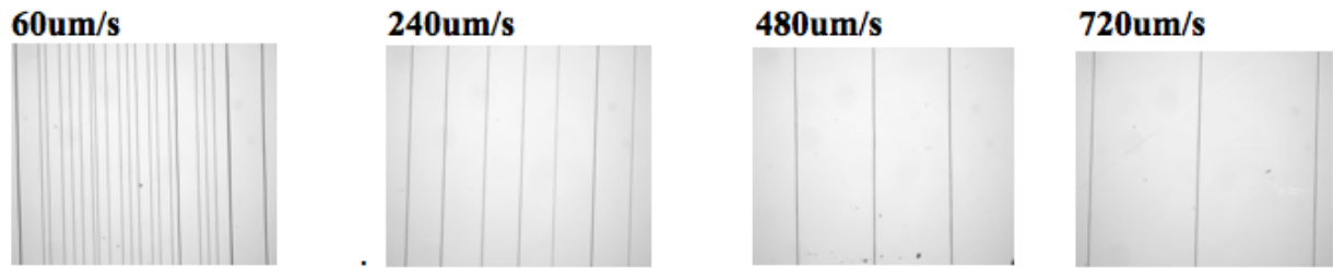
Figure 40: Some selected images of fibers obtained at various stage speed
