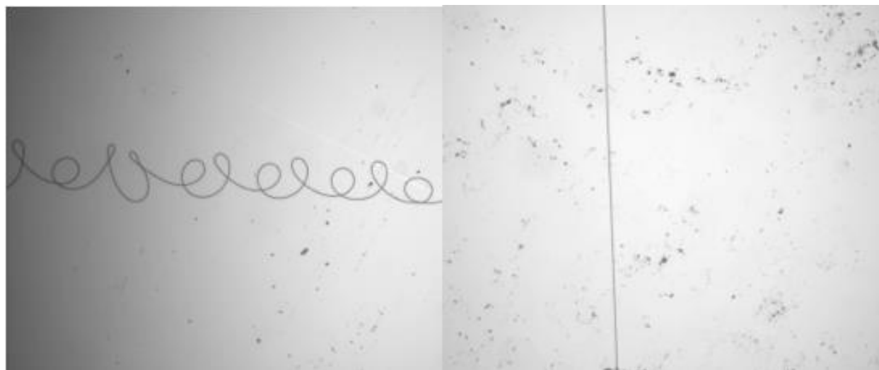
Figure 29: The nanofiber obtained by EMS (left) and new setup (right) at same applied voltage
