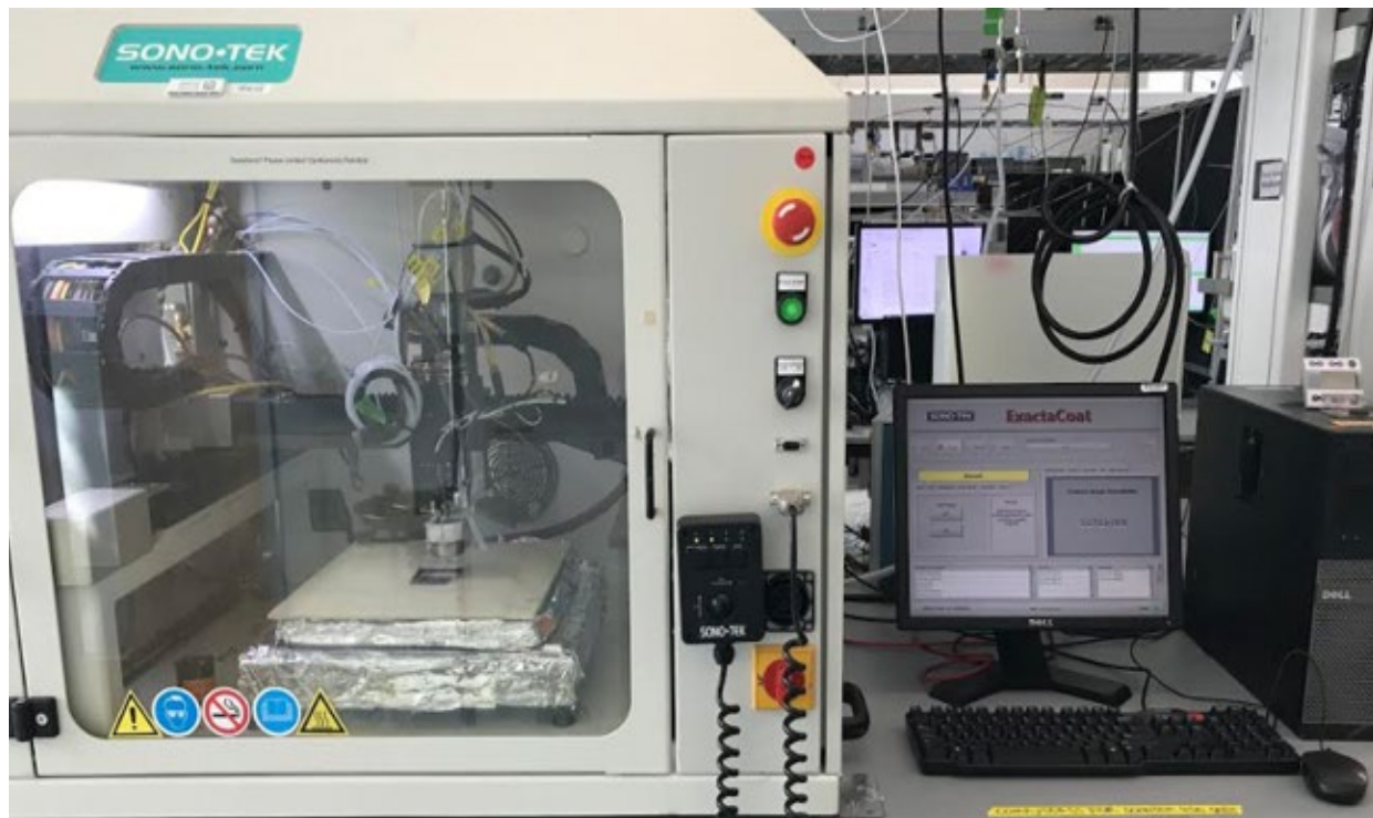
Figure 2.1. Sono-Tek ® spray coater test station used for MEA fabrication.
