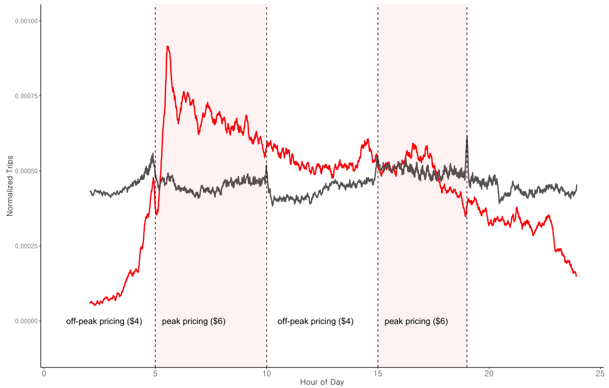
Figure A.6: San Francisco’s Bay Bridge imposed peak hour pricing on July 1, 2010 (see Section 1.4). This figure plots the density of passenger vehicle trips crossing the Bay Bridge in the hours surrounding each of the price notches in 2014 (records of cash payments are unreliable prior to 2014). The red line shows trips using an electronic FasTrak device; the grey line shows cash payments. This plot excludes trips that use the carpool lane, as well as eligible electric vehicles, each of which faced a different pricing scheme. The red shaded regions demarcate times of day that were subject to peak-hour pricing after July 1, 2010.
