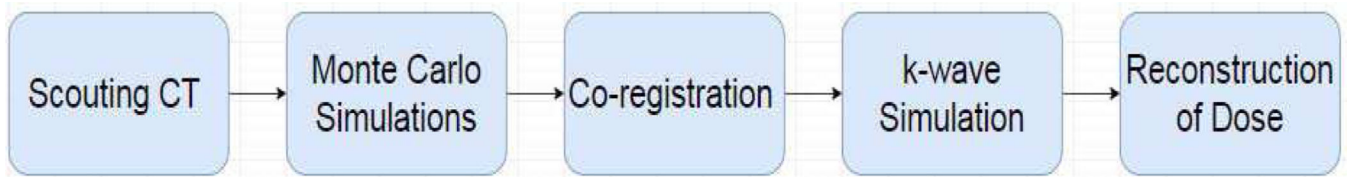
Fig. 2. Simulation Workflow for Protoacoustic Imaging
