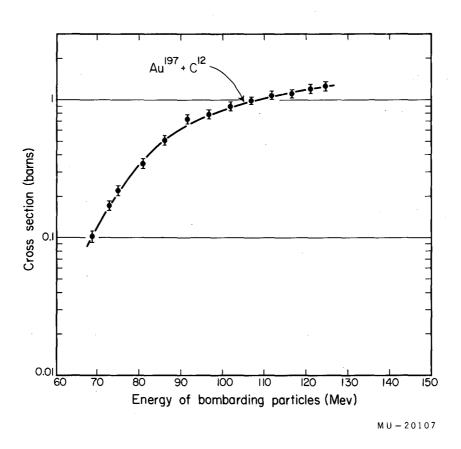
Fig. 8. Cross section for fission of  $\mathrm{Au}^{197}$  induced by  $\mathrm{C}^{12}$  ions as a function of bombarding energy.
