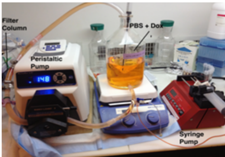
Figure 10: The set-up of the flow model that simulates blood flow in vitro .
