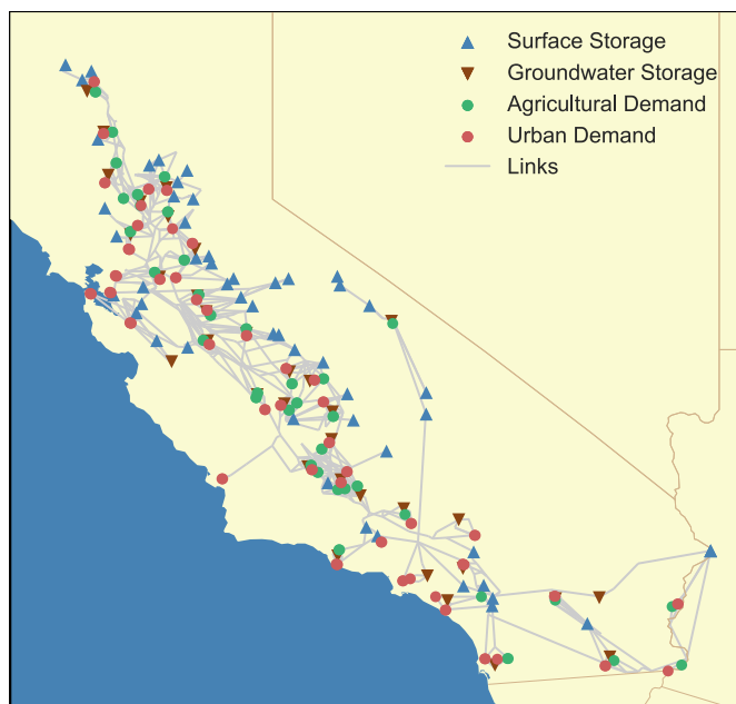
Fig. 1. Network representation of California's water supply system in the CALVIN model. Selected node types are shown; other node types include pumping plants, water treatment plants, and junctions.
